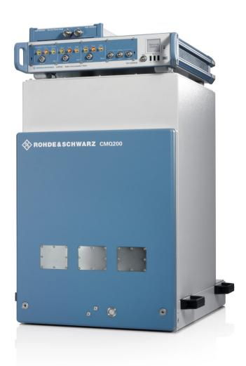
The split concept is a key feature of the one-box tester. The R&S°CMP200 can generate and analyze IF frequencies from 6 GHz to 20 GHz directly at the output. In higher frequency ranges, R&S°CMPHEAD30 seamlessly takes over this function.
