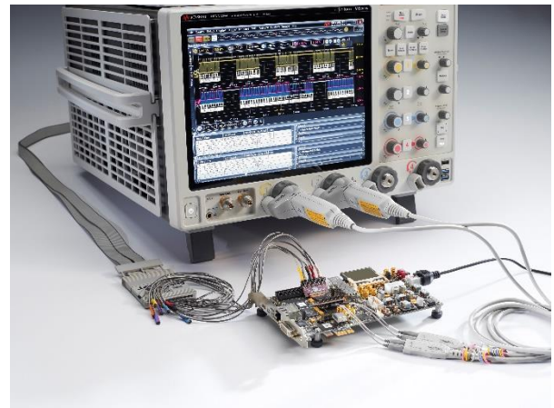
DDR3 test setup with mixed signal oscilloscope.
