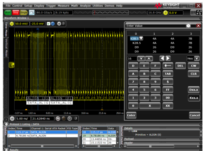
The V-Series' 8b/10b hardware triggers at 16 "K" and "D" symbols of the SATA signal. The software protocol decoder further decodes the symbols into higher-level data packets such as the SATA ALIGN packets.
