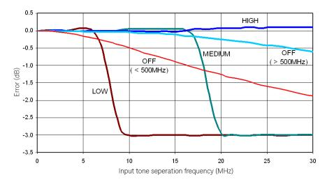
Figure 2. N192XA Error in peak-to-average measurements for a two-tone input (High, Medium, Low or Off filters)
