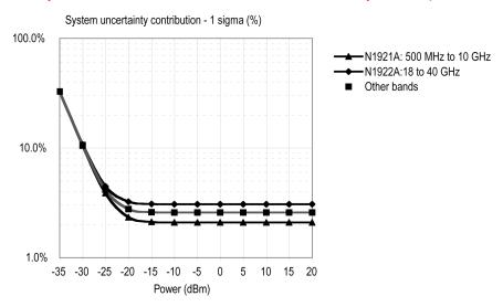
Note: This graph is valid for conditions of free-run operation, with a signal within the video bandwidth setting on the system. Humidity < 70%.
