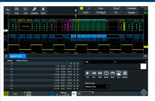
Use the digital channels to decode parallel buses. These are displayed in a digital bus format or as an analog waveform. For clocked parallel buses, the decoded contents can also be displayed in a table. In addition, you can use the digital channels of the R&S®RTx-B1 option to decode serial interface protocols such as SPI and I<sup>2</sup>C.
