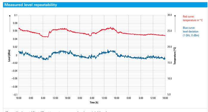
Measured level repeatability at different temperatures over a very long time period of three days. The graph shows the accuracy with which a 0 dBm level at 1 GHz is repeated (another level is always selected between two 0 dBm settings).
