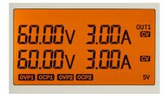
Figure 2. Backlight on/off feature with dual reading (voltage and current) on an LCD display
