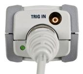
The external trigger input port on the U8481A.
