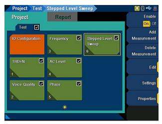
Figure 10. The test sequence control function comes with a selection of pre-configured measurements. It allows users to select the most frequently used test sequences for their daily measurement.
