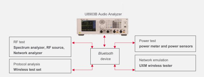
Figure 4. Total Keysight Bluetooth solution.
