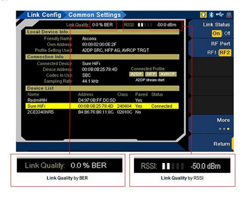
Figure 2. The bit error rate (BER) measurement and the received power indicator (RSSI) functions help ensure the quality of your *Bluetooth* link.
