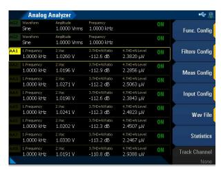
Figure 5. The U8903B's GUI, showing 8 analyzer channel measurements.
