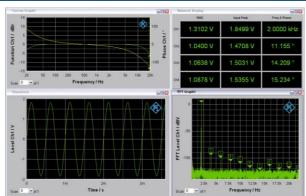
Everything at a glance: Multiple measurement diagrams can be arranged in any desired configuration on the screen; analyses in the frequency and the time domain can be displayed simultaneously.
