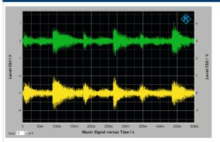
Complex test signals from WAV files can be output at all interfaces; in this example, the waveform function shows the time characteristic of a dualchannel music signal.
