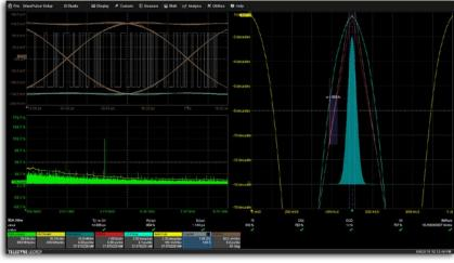
Complete Jitter Analysis including ISI eye-diagram.
