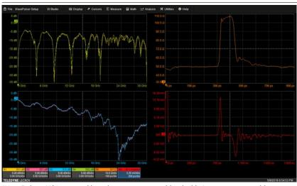
WavePulser 40iX step and impulse response combined with S-parameters enables determination of the type of impairment.
